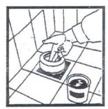
3. Incase of the usage at eccantrical pipe, soap should be applied to the joint parts of the pipe.
