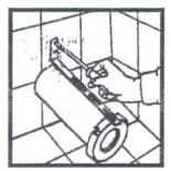
2. If the drainege is from wall, straight PVC Pipe should be used together with "L" fixing element and the metal ring.
