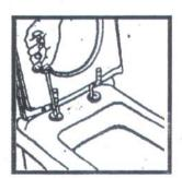
13. The seat cover should cover should be assembledto WC pan.
