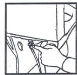
8. The clean water pipes should be assembled and be checked carefully incase of leakage.
