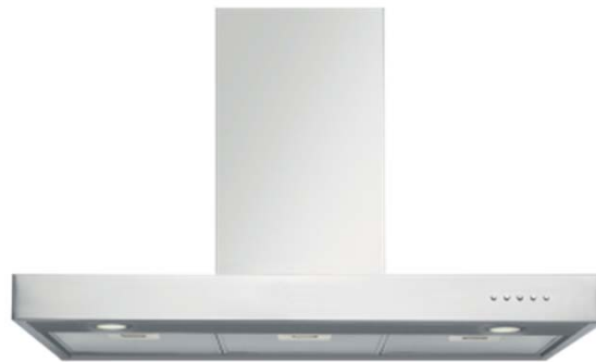
GEH9023 90CM SLIMLINE CANOPY RANGEHOOD 750m 3 /h, 3 Speed Fan 2 x Halogen Lights 3 x Aluminium Filters 1,200mm Flue Cover 150mm Ducting Outlet
